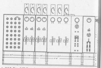
A-C.G.E. Type, 0-100 Range Ammeter, or Weston Model 24, 0-100 Range Ammeter. A 1-Weston Model 24, Range 0-300, Type No. 06505 or C.G.E. Type Range 0-300 Ammeter. R-C.G.E. Iron Grid Rheostat DL 174717 Form CR 9200. Capacity 60 Amps., 19 0h 115 Volts.
