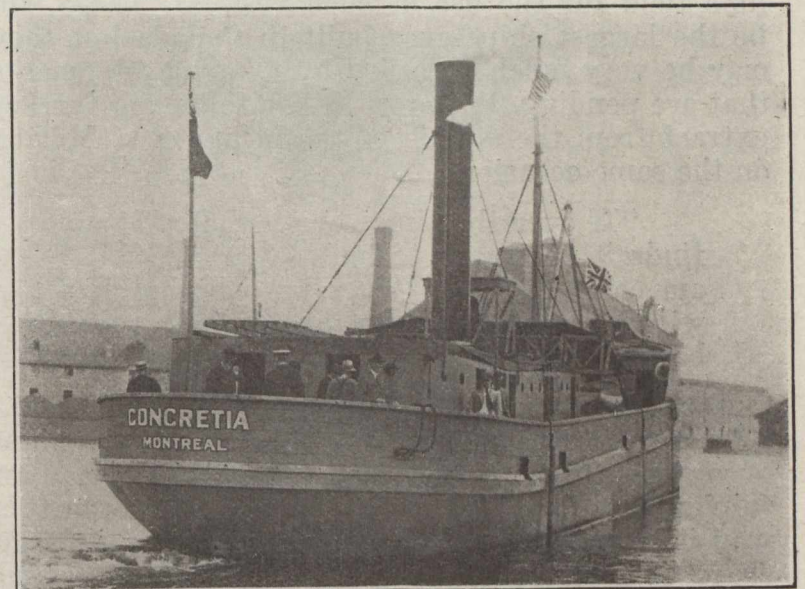
S.S. "Concretia," the first concrete ship built in Canada, designed by Mr. Thomas Hall, President of the Hall Engineering Company of Montreal. This vessel has since been bought by the Canadian Government for coast and river patrol service.
