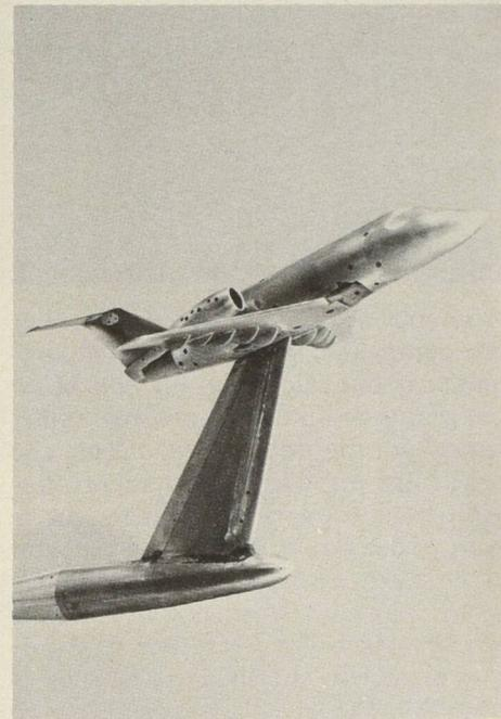
Tests on scale models of the Challenger were done at NRC's wind tunnels operated by the National Aeronautical Establishment. Altogether, it took 1,800 hours of wind tunnel time to arrive at the final configuration, a design close to aerodynamic perfection.
