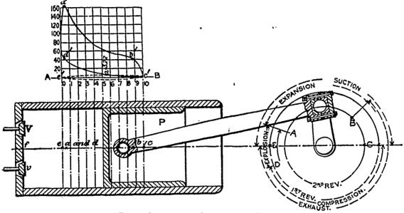
Fig. 1-Showing the Action of the Engine.
