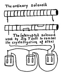
solenoid, on the contrary, whose curve is interrupted, carries a current which changes with the frequency of the interruptions, and has peculiar effects on metal placed within it. It induces in the metal, independently of the extreme poles, as many interior poles as there are alterations in the coil.
