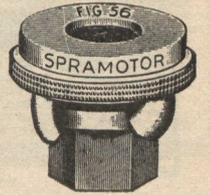
This illustrates the Spramotor Nozzle, Fig. 56, designed to apply lime sulphur mixture. It is made in brass with brass or steel removable discs, or with aluminum cap and body, and brass or steel discs. The particular merit of this type of nozzle is in the large liquid ways that prevent clogging and the double ways being at an angle that gives the most perfect form of spray.
