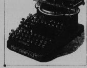
which is admirable both for its simplicity and the impossibility of getting out of adjustment. A line can be written clear to the bottom of the paper.
