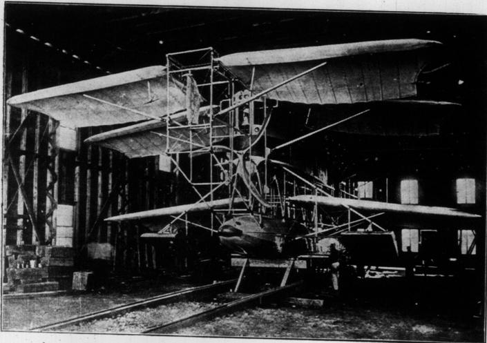
The mysterious twelve-winged craft, built in Savannah, Ga., which is expected by its inventor, Capt. Matthew A. Batson, of the U.S. Cavalry, to cross the Atlantic. It is a triple-motored multiplane with a speed capacity of from forty-five to sixty miles an hour on water and one hundred miles an hour in the air. It is seventy-four feet long and weighs about 9,000 pounds. The present plan is to make a preliminary flight from Savannah to New York, and then to try to cross the Atlantic.
