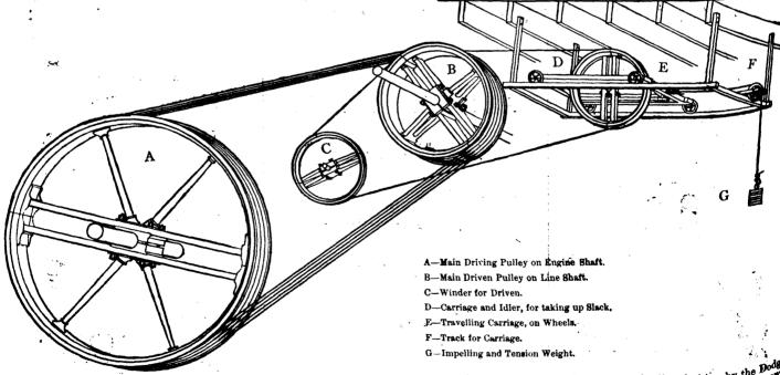
The illustration, as shown above, is one of peculiar construction, and represents an engine transmitting its power to the line shafting by the power to the line shafting by the
