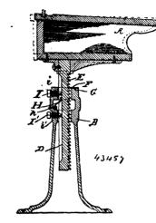
stantially as and for the purpose specified. 3rd. The combination of the stationary standard, formed with an annular recess in its interior, the vertically movable support sliding loosely in said standard, a friction or clamping spring consisting of a split ring located within the annular recess in the standard and adapted to press or bear against the movable support and the binding screws, substantially as set forth.
