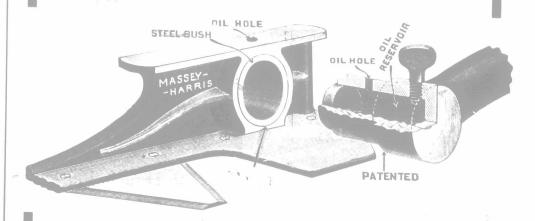
The oil is drawn up by suction through the oil hole by the natural action of the Pitman.
