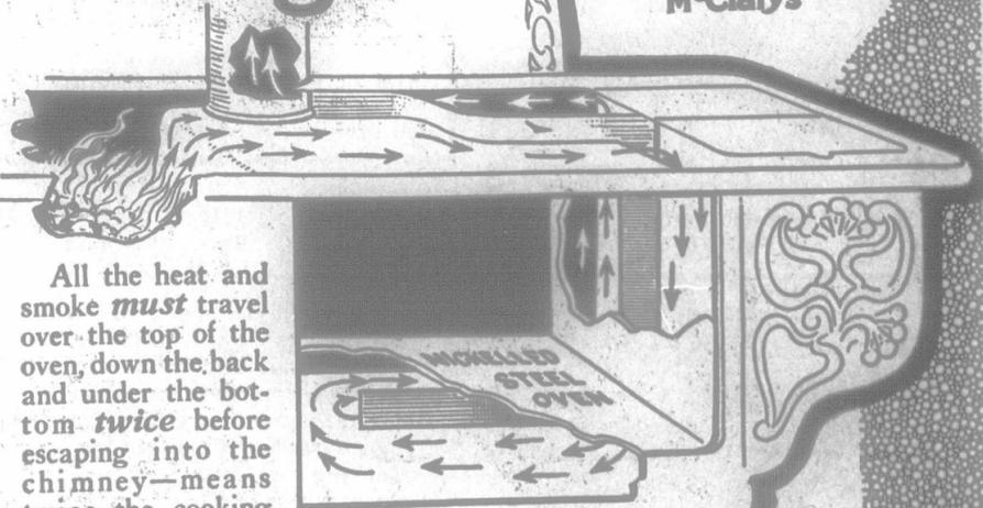
All the heat and smoke *must* travel over the top of the oven, down the back and under the bottom *twice* before escaping into the chimney—means *twice* the cooking and baking powers from the same amount of fuel as given by the ordinary range.
