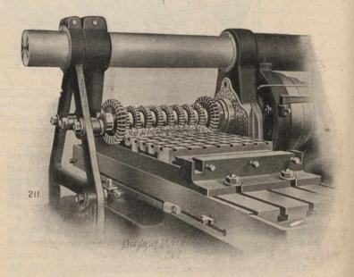
work on these pieces as they are finished now. The actual time required is two hours for each plate, just one-ninth of the time formerly required, and when the pieces leave the miller, they are accurate and go together nicely.
