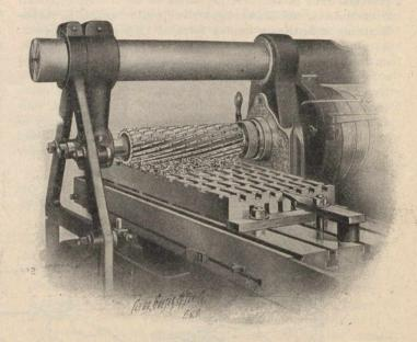
grooves are finished out to size, and the edges of the piece are squared up. R. P. Deardorff, who had charge of this work at the time the photographs were taken, stated that the chief thing about the plates is the accuracy required, it being highly desirable that the plates go together accurately without any hard-fitting.
