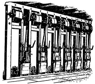
When two or more knives are n with one belt, all must stop when the belt is stopped to set bits or from ar other cause. Our Machine has a be for each knife, hence but one kni stops at a time. This great advantage should not be overlooked by purchasers. Time is money. Our Machin cuts more excelsior in a given tin than any other machine. Get of circulars and prices.
