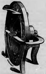
WHEEL JOINTER FOR SHINGLES AND HEADING. This engraving represents my Iron Wheel Jointer for Jointing: gen pate Wh
