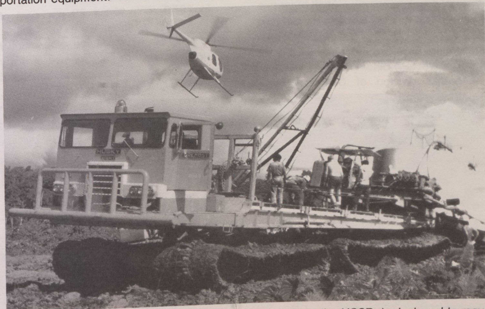
The large Husky-8G four-tracked vehicle, recently sold to the USSR, is designed to move heavy payloads in mud, muskeg, swamp, and snow conditions. The independent crankarm suspension and flexible track provide constant ground contact, absorb shock loads and increase productivity by allowing higher travel speeds than steel tracks.
