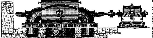
HE accompanying cut shows the direct con-nection of two 20' CROCKER TURBINES under 50 ft. head to ELECTRICAL GENERATOR at power station of North Shore Power Co., at St. Narcisse, Que. Two sets were furnished
