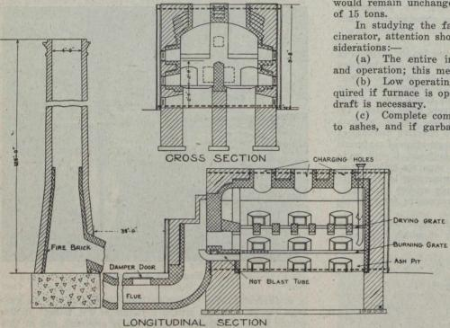
The cells of the furnace are so arranged that entrance can be had to each cell at each different chamber by means of outer doors. The entire furnace is supported on reinforced concrete footings.
