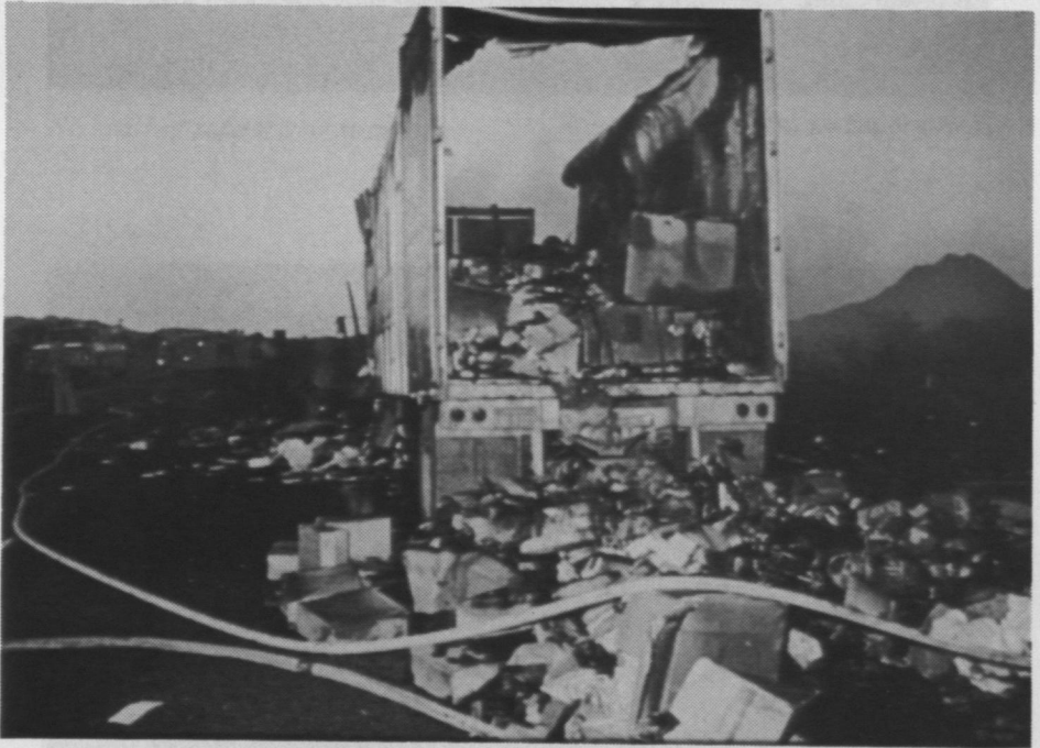
Explosion from friction by loose cargo
