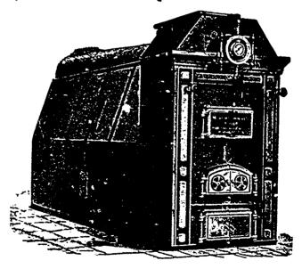
Has internal fire-box. Water circulation similar to a Water Tube Boiler. Large heating surface, and special arrangements for preventing and removing scale. Tests show high economy. Built with sheet steel case, or for brick casing, as desired.
