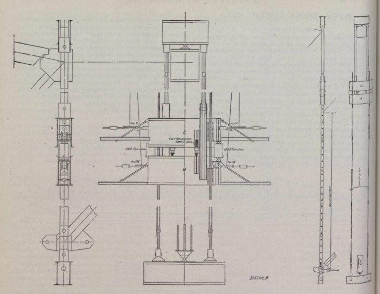
so that the valve operators at the corners may keep the moving girder C exactly horizontal and the valve operator at the centre of the span may keep the span itself horizontal. A telephone system has been arranged by which each lift at the ends of the span will be reported to the officer in general charge and the two ends thus kept at the same vertical height.
