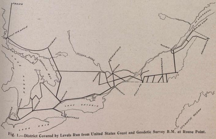
accumulation of errors on long lines. One of the most important precautions is the system of duplicate levelling all work being run at least twice, in opposite directions.  $T_0^{all Work}$  being run at least twice, in opposite under the set of ordinary levelling various will reveal themvarious other differences in procedure will reveal them-selves during the course of this paper.
