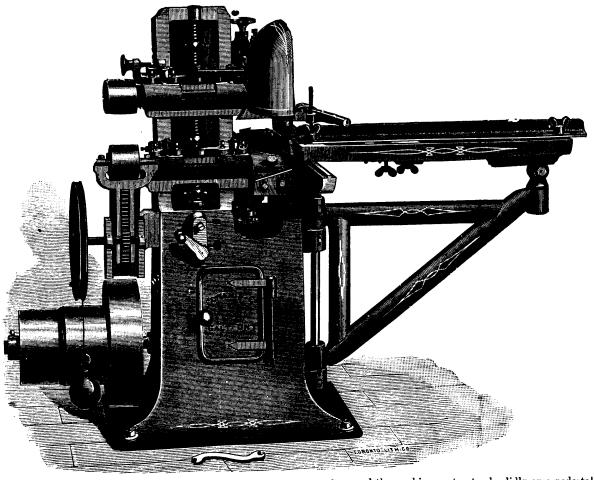
This is an entirely new style of Tenon Machine. The frame is cast in one piece, and the working parts stand, solidly on a pedestal, avoiding vibration,
