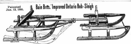
Best Sleigh in the Market! Because it is the lightest running, shortest turning; never cuts off; is always in line; no wearing of box or rack; no splitting of bolster or reach; never buckles; can be backed like a wagon; built of the very best material; strong and durable.
