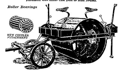
With Roller Bearings and New Patent Coupler Attachment, either 2½, 3½, 4½ or 5½ tons. All one size frame, drum, and width of tread and can be extra weighed 2 tons each. Address for Catalogue
