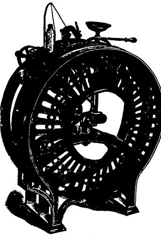
The Rayer and Liucoln Combined Sewing, Tromag and Stamping Machine is, if desired, supplied without marking along at reduced price. It sews the piece ends and cuts off the raw aloges. This is the simplest make of this machine, having no complicated and elaborate mechanism for stripping the cloth. Repairs are therefore reduced to a minimum. Made by W. H. Harrap, Richmond Hill, Blackfriars street, Salford, Manchester.
