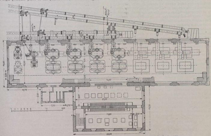
Fig. 6.—Plan of Isola Power House, Showing Distributor Pipes Scale 1: 400.
