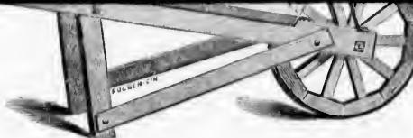
Same as Ore Barrow, except the tray, which is shaped specially for the purpose, and is 10 inches deep at handles and 13 inches at wheel; bottom, 19½ inches square; top, 27 inches wide by 29 inches long. Edges of tray iron strapped. Weight, 55 lbs.
