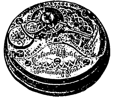
16 Size, Nickel.—No. 34, Hunting, or No. 95, Open Face, pendant set, 15 jewels, adjusted, jewels set in gold, Breguet hair spring, sunk seconds dial.
