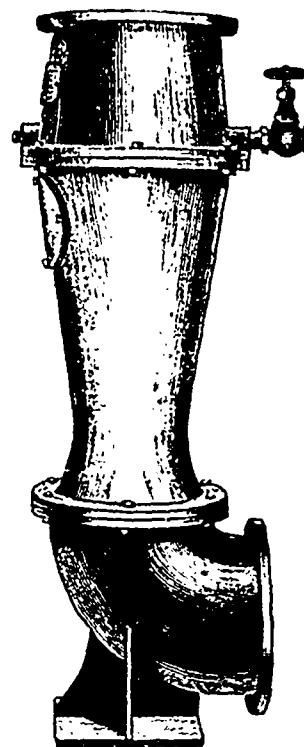
FIG. 3.—UPRIGHT COMBINED AIR INJECTOR AND EXHAUSTER
