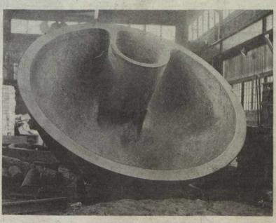
SMELTER LEAD POT-18,000 Pound Steel Casting
