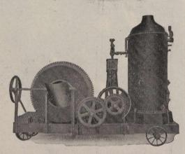
We supply Ransome Mixers, in all sizes, equipped with styles of power.
