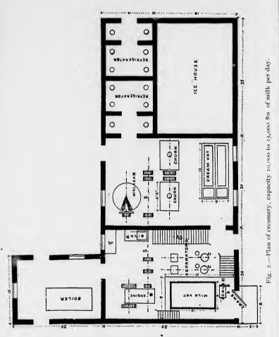
The refrigerators occupy two stories. The upper story comprises a room which communicates by a stairway on one side with the garret of the factory and on the other side by a door with the ice house. The cylinders in the lower rooms open into it. In this room the ice is broken up before being placed in the cylinders. This will be treated of later on.
