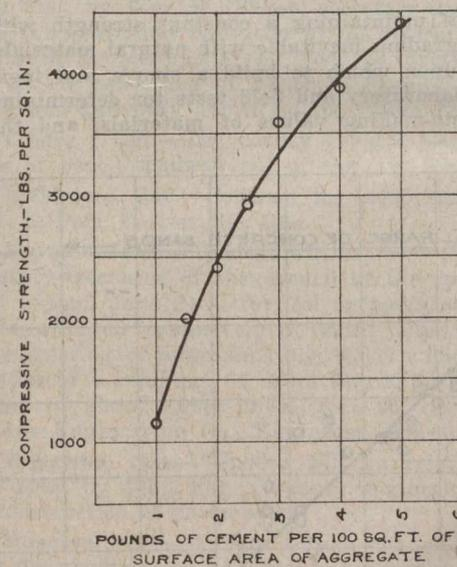
FIG. 6—RESULTS RECENTLY OBTAINED IN THE "HYDRO" LABORATORY
