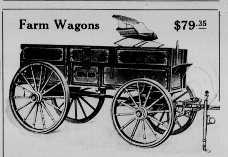
Here is the Abingdon Wagon recognized as one of the best manufactured anywhere. It is built of select-stock hickory and white oak.  $3\frac{1}{4} \times 10$ , 3 in. tire, complete with trees, neckyoke and spring seat, with 28 in. box. Weight 1,150 lbs.
