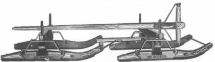
BOLSTERS are equipped with iron stakes—fastened with bolts and rivets to prevent ends of bolsters from splitting. ROLLER RODS for tongue and reach are full length. BOLSTER PLATES large and made of steel. START PINS are \( \) in., plates rivetted
