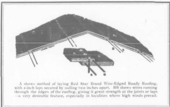
A shows method of laying Red Star Brand Wire-Edged Ready Roofing, with 2-inch laps secured by nailing two inches apart. BB shows wires running through the edges of the roofing, giving it great strength at the joints or laps—a very desirable feature, especially in localities where high winds prevail.
