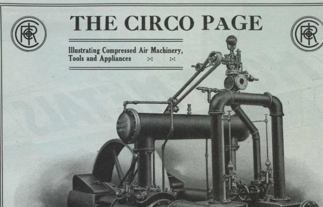
Class "RL-3" Duplex Type, Steam Driven Air Compressor, with Cross Compound Steam and Cross Compound Air Cylin-ders with Intercooler. Machine is convertible to Belt Drive when required, and is equipped with Speed and Pressure Governor, "Circo" Silent Leaf Inlet and Outlet Valves, Enclosed Dust-Proof Construction, Splash Lubrication System and Meyer Adjustable Cut-off.
