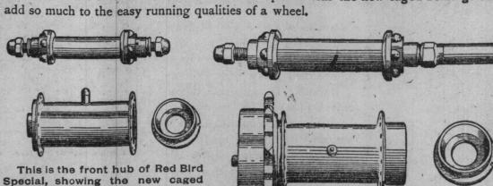
Rear hub of Red Bird Special, showing Wilson automatic brake and new caged bearings.
