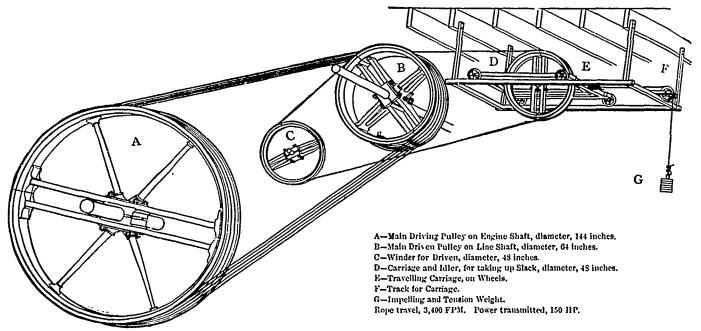
The illustration, as shown above, is one of peculiar construction, and represents an engine transmission of power by a manilla rope, under the Dodge system of patents, and is shown as in actual use at the works of the Dodge Mfg. Co., at Mishawaka, Ind.
