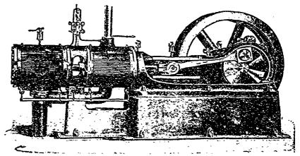
In the TANDEM COMPOUND the High Pressure Cylinder is placed next the frame, and both Pistons and Cylinder ' Heads may be withdrawn through the Low Pressure Cylinder without disturbing it. Both Valves are controlled by the Governor, so arranged that an equal amount of work is done in each Cylinder.
