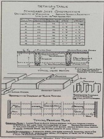
Diagram Showing Joist Construction.
