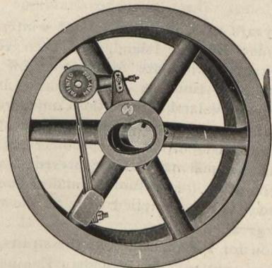
“Straight Line” governor. The result is an extremely simple and powerful governor, in which there is not enough friction to prevent it from changing position almost instantly to meet sudden changes of load, and there is no possibility of racing when properly adjusted. By means of a simple adjustment of the link connecting the eccentric and centrifugal weight, the governor weight may be adjusted to any degree of sensitiveness or close regulation. Only an engineer who has had experience
