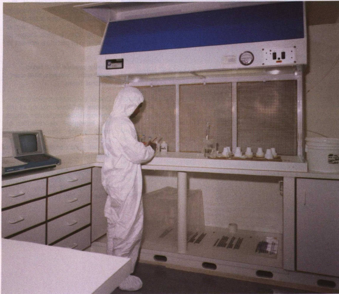
Class 100 Clean Room for the determination of trace levels of environmental contaminants.
