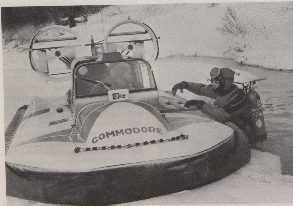
Jeff Stephenson (right), a member of the National Association for Search and Rescue, and Colin Knight, are studying the use of hovercraft in the frigid -20°C waters of the Assiniboine River near Headingly, Manitoba. Mr. Knight designed the hovercraft for rescues on thin ice and open water when other methods are impossible.
