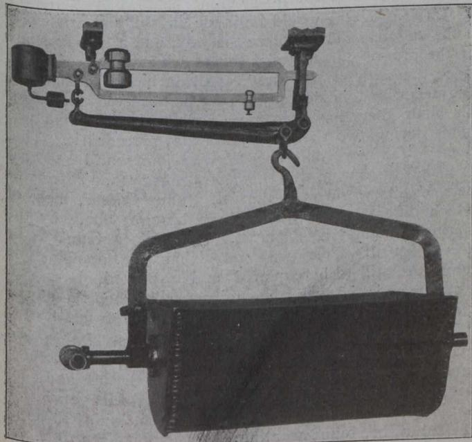
Fig. 8.—Asphalt Weighing Bucket
