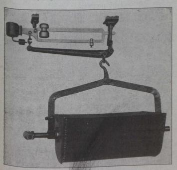
Fig. 8.—Asphalt Weighing Bucket
