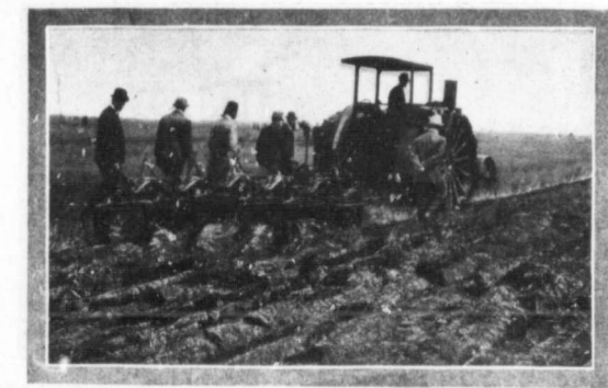
The Avery Gasoline Tractor pulling a Five Bottom Avery Self-Lift Plow. (Bronze medal winner Class B.)
