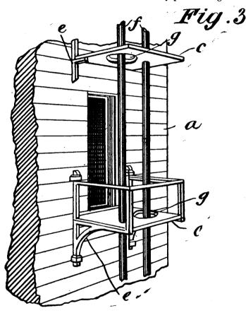
floors or staging from the root to the ground; g g are c cular openings which alternate from one side to the other at each succeeding landing. The landing to be placed before a window at every story.
