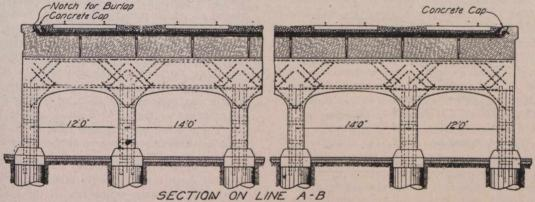
Fig. 8. Standard Method of Waterproofing Subways; C. B. & Q. Track Elevation Work, Chicago.
