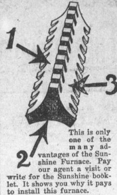
Note the three surfaces, each of which will last as long as the ordinary one surface grate. A gentle rocking is usually all that's required but any clinkers happening to form are ground up by the massive teeth of the four grates with very little effort. The grate bars are so constructed that a volume of air passes freely to all parts of the fire.
